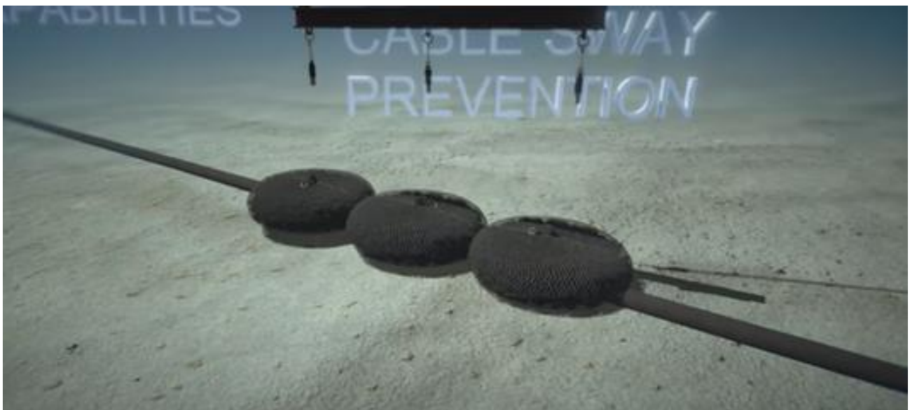
Plate 4-14: Example illustration of rock bags used for cable protection in the transition zone
