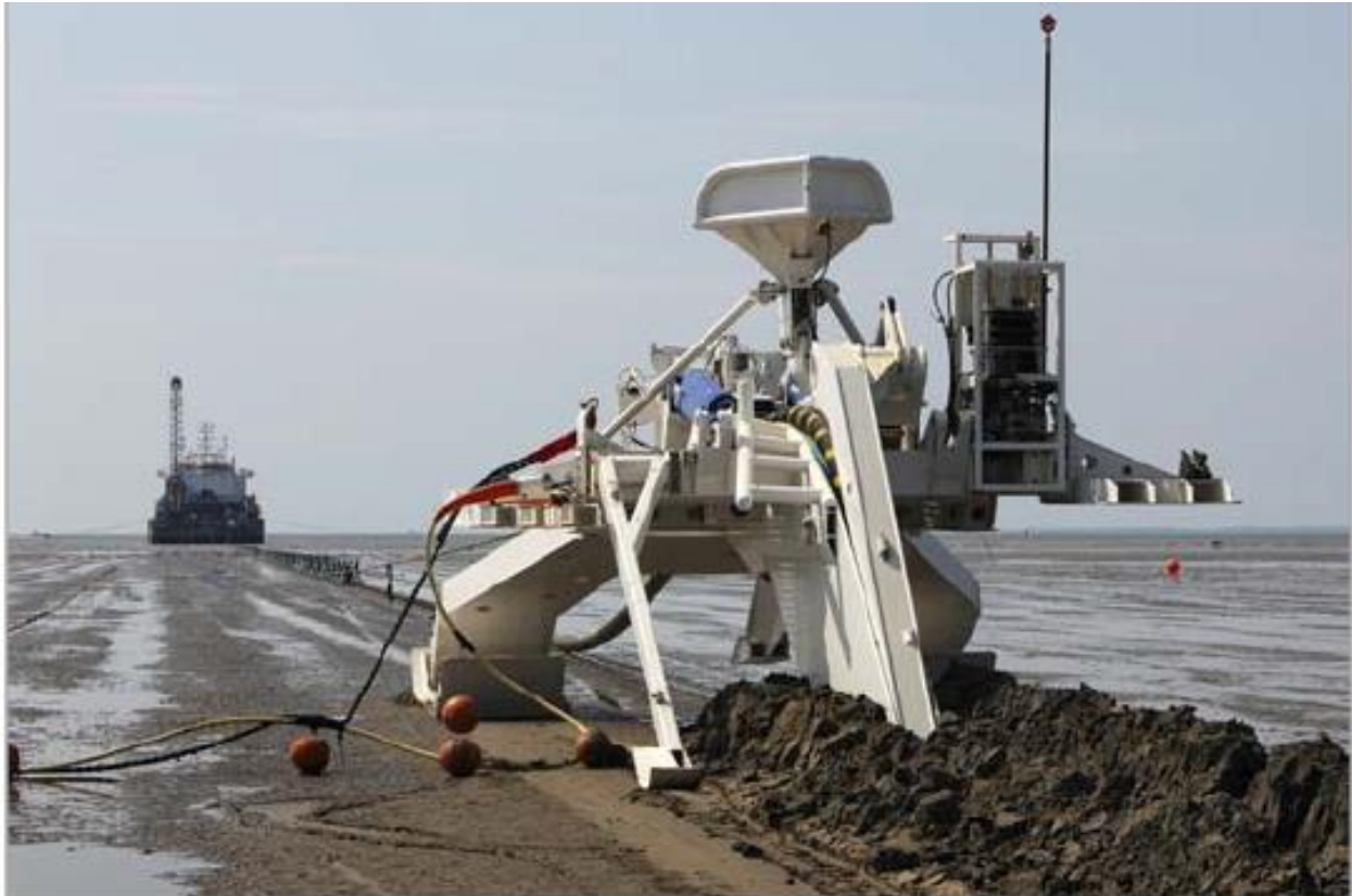
Plate 4-10: Example of a non-displacement plough (Source: Equinor)
